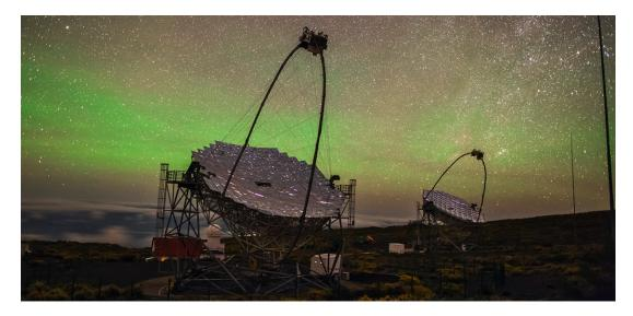
**Figure 1:** The MAGIC stereo system composed of two 17 m diameter dishes operating simultaneously. Telescopes are located in the Roque de los Muchachos Observatory in the Northern Hemisphere (28.7°N, 17.9°W). Courtesy of D. Lopes (IAC).
