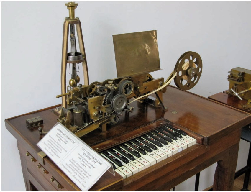
FIGURE 3 – The letter-printing telegraph set built by Siemens and Halske in Saint Petersburg, Russia, ca. 1900, based on the 1855 patent of David Hughes. (Source: Wikimedia Commons.)
