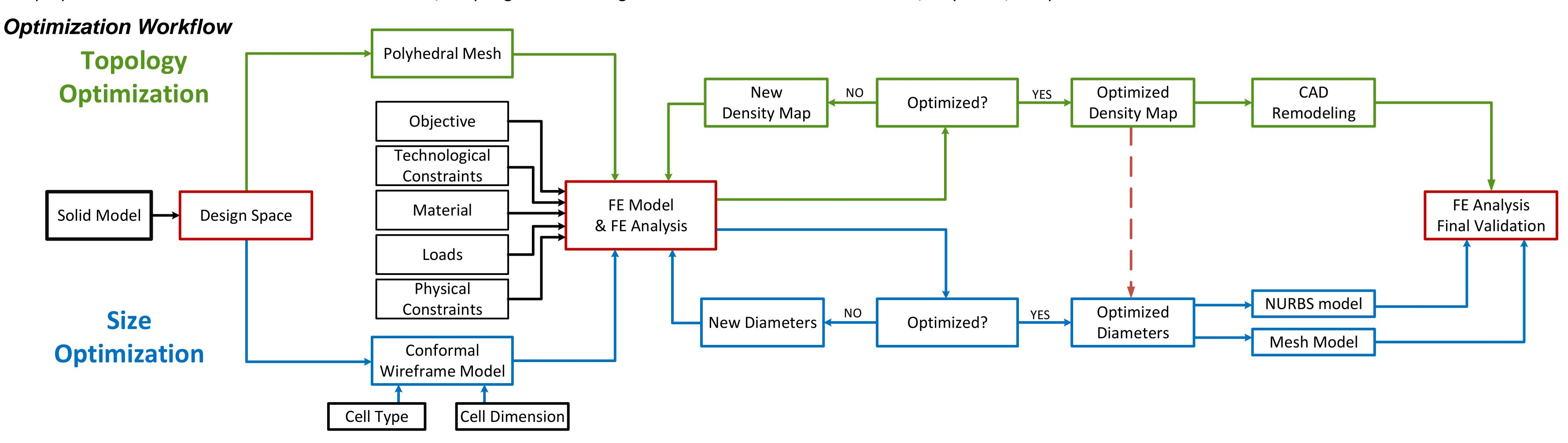
Topology optimization  $\rightarrow$  material is arranged in order to find the best distribution under a set of boundary conditions and respecting the structural and dimensional performances requirements. The goal of the optimization can be to maximize the stiffness, imposing a desired reduction of mass; these targets are reached varying the density of each element of a polyhedral mesh, which is related to the mechanical properties.
