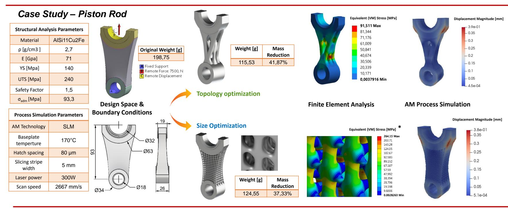
The results reported in the table show the similar percentage of mass reduction obtained with these two methods applied to a piston rod.
