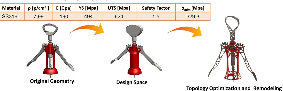
Topology optimization can be applied to assembly. In the corkscrew case, the topology optimization is performed taking into account both external loads and internal ones generated from contact points.
