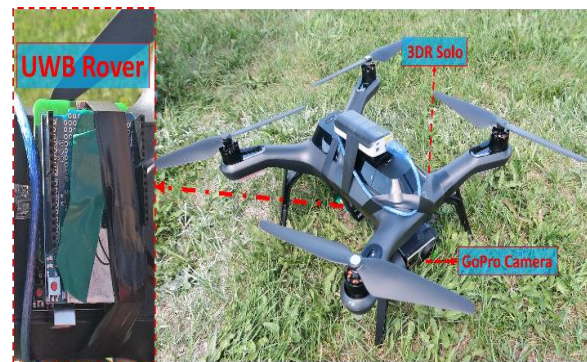
Figure 2. 3DR Quadcopter with UWB system and camera attached to it.
