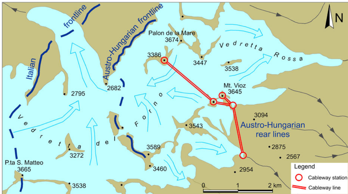
Fig. 2. Schematic map showing the frontline established in 1915 and the cableway system connecting Austro-Hungarian rear lines to the frontline.
