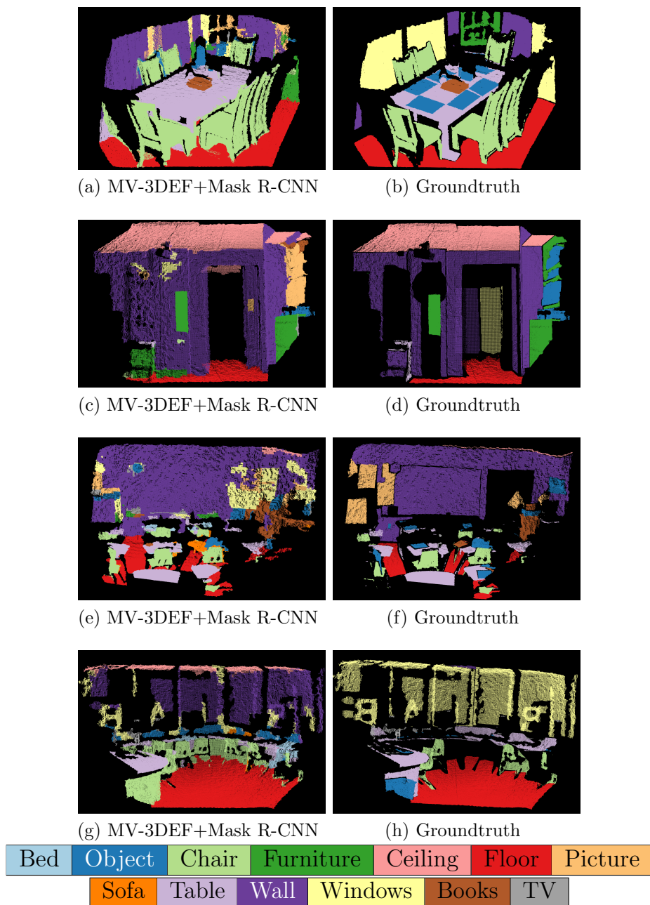
Figure 10: Qualitative results on the NYUv2 dataset: (a)(c)(e)(g) multi-view semantic segmentation obtained with the best of our methods, MV-3DEF+Mask R-CNN and (b)(d)(f)(h) groundtruth semantic segmentation.
