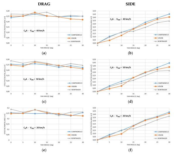
**Figure 5.** (**a**,**c**) Drag and (**b**,**d**) side effective frontal areas of the three wheelsets varying the yaw angle  $\beta$  (by 5° increments) with a constant wind speed referred to the bicycle VwB of 40 km/h and 50 km/h; (**e**) drag and (**f**) side effective frontal areas of the three wheelsets varying the yaw angle  $\beta$  (5° increments) with a constant wind speed referred to the ground VwG of 20 km/h.
