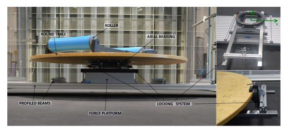
Figure 1. Front view of the supporting system with all the parts and details of the locking system.
