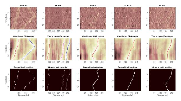
**Figure 6.** Tracking examples for several TD matrices featuring multiple and single moving targets, at different levels of Signal-to-Clutter ratios. The top row shows the input (noisy) images. The middle row shows the CDA (denoised) images, with the tracked path discovered by our CDA-TBD algorithm superimposed as a red curve. Bottom panels show the corresponding ground truth position of the targets.
