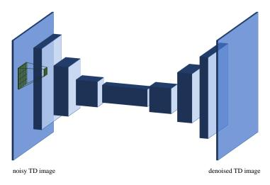
**Figure 4.** Diagram of the Convolutional Denoising Autoencoder (CDA). The noisy TD image is given as input and processed by a stack of convolutional layers, which detect increasingly more complex features in the signal that are then used by the decoder to produce a denoised TD matrix.
