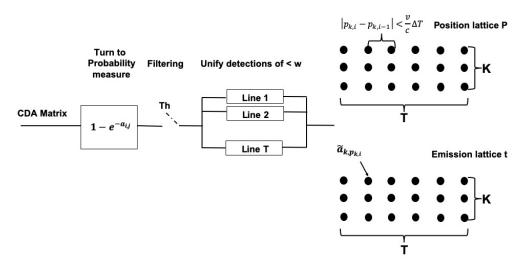
Figure 5. Block diagram for the processing of the CDA matrix before dynamic programming-based tracking.
