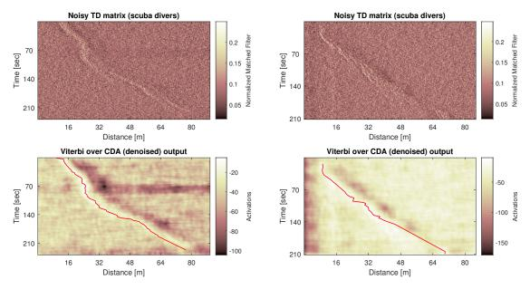
**Figure 7.** Application of the proposed methodology to TD matrices recorded from the movement of scuba divers.
