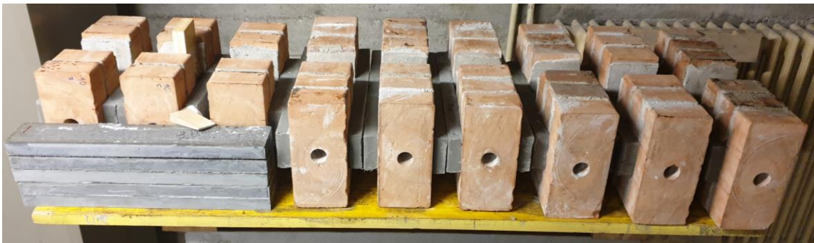
Fig. 12. Double shear lap test specimens.
