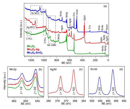
**Figure 3.** (a) X-ray photoelectron spectroscopy (XPS) wide-scan spectra pertaining to bare  $Mn_3O_4$ ,  $Mn_3O_4$ -Ag and  $Mn_3O_4$ -SnO<sub>2</sub> samples. (b) Mn2p, (c) Ag3d and (d) Sn3d photoelectron peaks. The color code is reported in panel (a).
