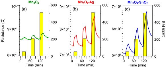
**Figure 6.** Dynamical responses of  $Mn_3O_4$  (**a**),  $Mn_3O_4$ -Ag (**b**) and  $Mn_3O_4$ -SnO<sub>2</sub> (**c**) nanosystems vs. different  $H_2$  concentrations, at a fixed working temperature of 200 °C.
