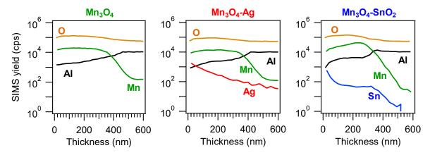
**Figure 4.** Secondary ion mass spectrometry (SIMS) depth profiles for Mn<sub>3</sub>O<sub>4</sub>, Mn<sub>3</sub>O<sub>4</sub>-Ag and Mn<sub>3</sub>O<sub>4</sub>-SnO<sub>2</sub> specimens.
