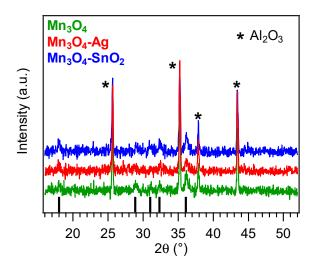
**Figure 2.** X-ray diffraction (XRD patterns for bare and functionalized  $Mn_3O_4$  nanosystems. Vertical black bars correspond to  $\alpha$ -Mn<sub>3</sub>O<sub>4</sub> signals [59].
