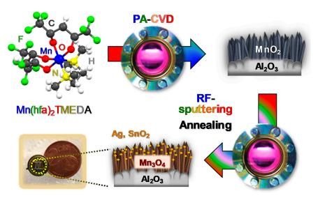
**Figure 1.** Scheme of the route proposed in the present study for the fabrication of  $Mn_3O_4$ -Ag and  $Mn_3O_4$ -SnO<sub>2</sub> nanomaterials.
