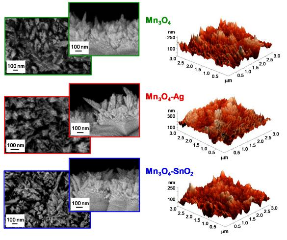
**Figure 5.** Representative plane-view and cross-sectional field emission-scanning electron microscopy (FE-SEM) micrographs (left panels) and atomic force microscopy (AFM) images (right panels) for Mn<sub>3</sub>O<sub>4</sub>, Mn<sub>3</sub>O<sub>4</sub>-Ag and Mn<sub>3</sub>O<sub>4</sub>-SnO<sub>2</sub> samples.
