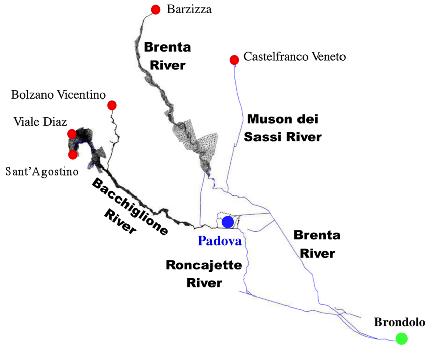
Fig. 3. Computational mesh used to model flood propagation in the Brenta-Bacchiglione river network. Red points denote inflow boundary conditions; the green point locates the Brenta mouth in the Adriatic Sea at Brondolo.
