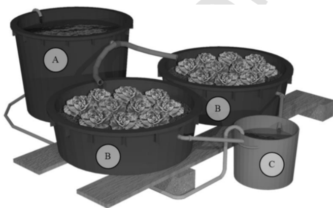
Fig. 1. Rendering of the aquaponic unit. A, main tank for fish (500 L); B, tanks for vegetables/biofilters (275 L); C, storage tank for water collection (50 L) and pumping to A tank.
