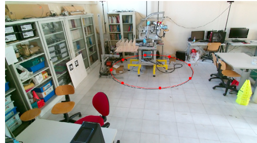
Figure 6. Experimental testbed in our lab. The red circle on the floor represents the danger zone obtained in the calibration step.
