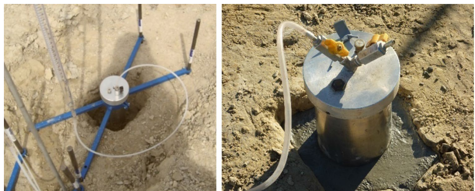
Fig. 12 Boutwell permeameter tests
