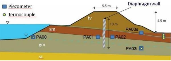
Figure 1. Schematic section of the monitored levee
