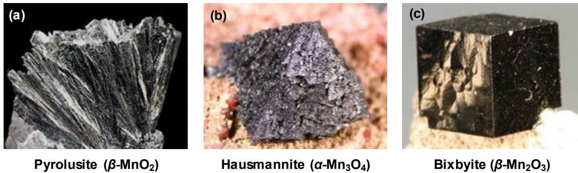
Figure 1.1.1. Picture of (a) pyrolusite ( \beta -MnO 2 ), (b) hausmannite ( \alpha -Mn 3 O 4 ), and (c) bixbyite ( \beta -Mn 2 O 3 ) ore. 46
