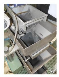
**Figure 15.** Case study hoppers cascade system. In this application the system is composed of three hoppers and a weighing device in the middle one.
