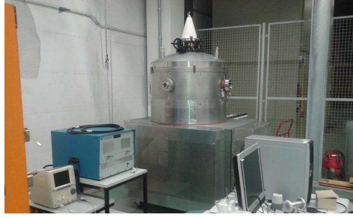
Figure 26. Final setup of the high voltage radio frequency test facility.
