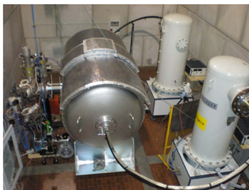
Figure 24. View of the HVPTF 800 kV setup. The tank with the lead screening on the top and the two \pm 400 kV/1 mA power supplies are shown. Connection to the electrodes is made via coaxial XLPE cables.
