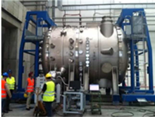
Figure 3. View of the SPIDER vacuum vessel during vacuum tests at the PRIMA site.
