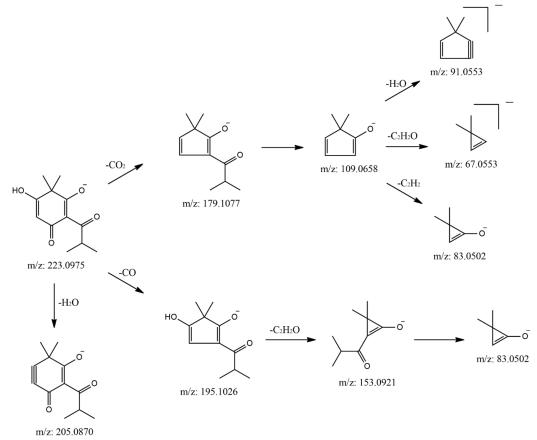
**Figure 4.** Proposed fragmentation scheme for 3'3'me6'oxoPIB,  $[M-H]^- = 223$ . The main fragments are shown together with information about their *m*/*z* values. The mass spectra with the peaks assignable to each fragment are reported in Figure 3.
