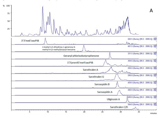
**Figure 2.** Representative chromatogram obtained from LC-ESI(-) ion trap analysis of *H. japonicum* extract (panel A) and extracted ion chromatograms of the characterized phloroglucinol derivatives. Each chromatographic trace shows the peak(s) associated with a specific phloroglucinol, whose name is indicated. 3'3'me6'oxoPIB: 3',3'-dimethyl-6'-oxo-phlorisobutyrophenone; 1'3' pren45'me4'oxoPIB: 1',3'-diprenyl-4,5'-dimethyl-4'-oxo-phlorisobutyrophenone.
