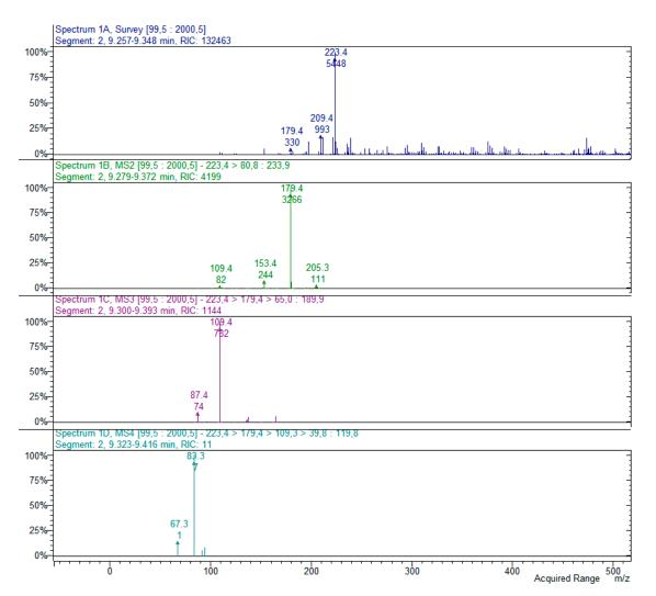
**Figure 3.** MS<sup>n</sup> spectra (n = 4) of 3'3'me6'oxoPIB, [M-H]<sup>-</sup> = 223. The spectra show the main fragments formed by the sequential fragmentation of the parent compound (m/z 223 > 179) and its main products (m/z 179 > 109; m/z 109 > 83). The structures of the main fragments are reported in the scheme in Figure 4.
