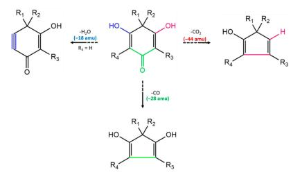
**Figure 5.** Characteristic proposed fragmentations for monomeric PIB derivatives. The "blue" path leads to the elimination of a molecule of water and to the formation of a triple bond. The "green" path leads to the elimination of a carbonyl group, with further rearrangement of the ring. The "purple" path leads to the elimination of CO<sub>2</sub>, followed by rearrangement of the ring.
