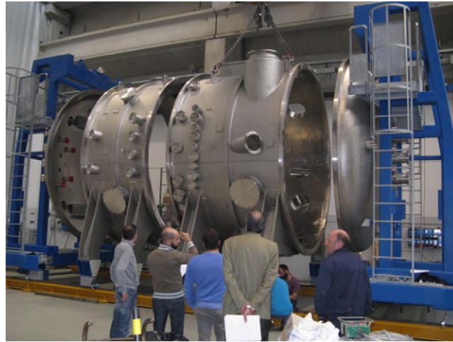
Figure 6. SPIDER vacuum vessel during assembly at supplier premises for factory tests.
