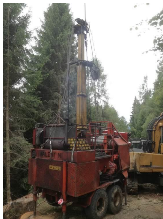
Figure 1: Cable yarder VALENTINI V850 M3.
