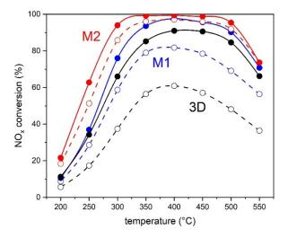
**Figure 8.** Maximum  $NO_x$  conversion (solid lines) and  $NO_x$  conversion at 10 ppm  $NH_3$  slip (dashed lines) of the three samples M1, M2, and 3D-printed.
