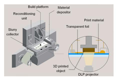
Figure 5. Schematic representation of the industrial ceramic 3D printer.
