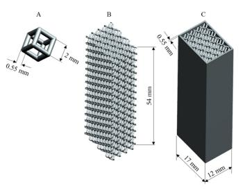
**Figure 4.** CAD file of the developed architecture: (**A**) rotated cube unit cell; (**B**) cell replication; (**C**) tubular lattice.
