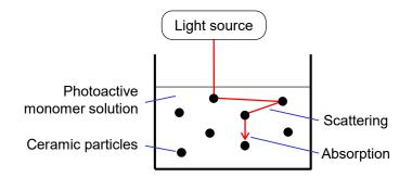
**Figure 1.** Schematic representation of the scattering phenomenon occurring when a ceramic slurry is invested by photons.
