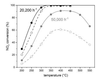
**Figure 9.** Maximum NO<sub>x</sub> conversion (solid lines) and NO<sub>x</sub> conversion at 10 ppm NH<sub>3</sub> slip (dashed lines) of sample 3D printed at GHSV = 50,000 h<sup>-1</sup> and GHSV = 22,200 h<sup>-1</sup>.
