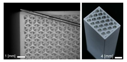
**Figure 6.** (left): 3D-printed closed-walls lattice, the base cells correspond to a rotated cube with a struts diameter of 0.20 mm, a cell length of 1 mm, and a wall thickness of 0.55 mm. As a reference, a sewing needle with a diameter of about 0.4 mm is placed on the component. (**right**): 3D-printed and sintered closed-walls lattice in its final configuration, the base cells correspond to a rotated cube with a struts diameter of 0.55 mm and a cell length of 2 mm.
