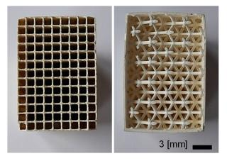
Figure 7. (left): washcoated cordierite honeycomb (M1); (right): washcoated 3D-printed alumina lattice.
