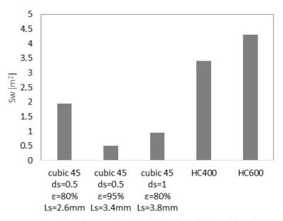
**Figure 2.** Wetted surface area ( $S_w$ ) by the gas flow of three additively manufactured structures based on a rotated cube elementary cell (cubic 45) for different struts diameter (ds), porosities ( $\epsilon$ ), and cell size (Ls) in comparison with two state-of-the-art honeycombs (HC) with different cpsi (i.e., 400 and 600). Data source [16].
