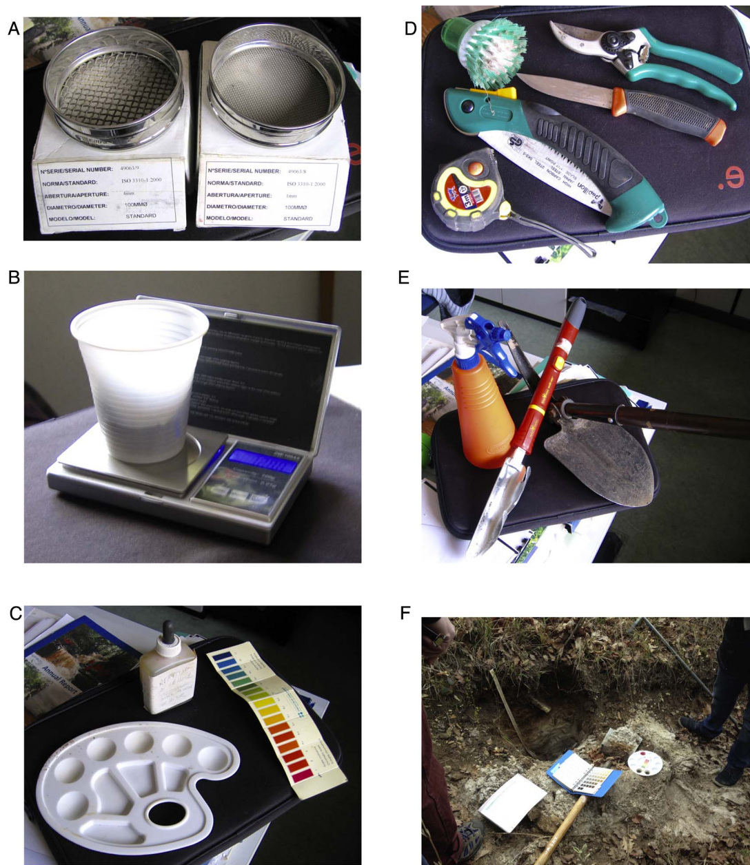
Fig. 13. Common tools used for field humus investigations: a) sieves (1 mm, 4 mm); b) digital scale for the estimation of weight (volume) of bio-aggregates; c) colorimetric estimation of \text{pH}_{\text{water}} ; d) and e) tools used for the preparation of humus profiles; f) field key of classification and Munsell soil colour chart.
