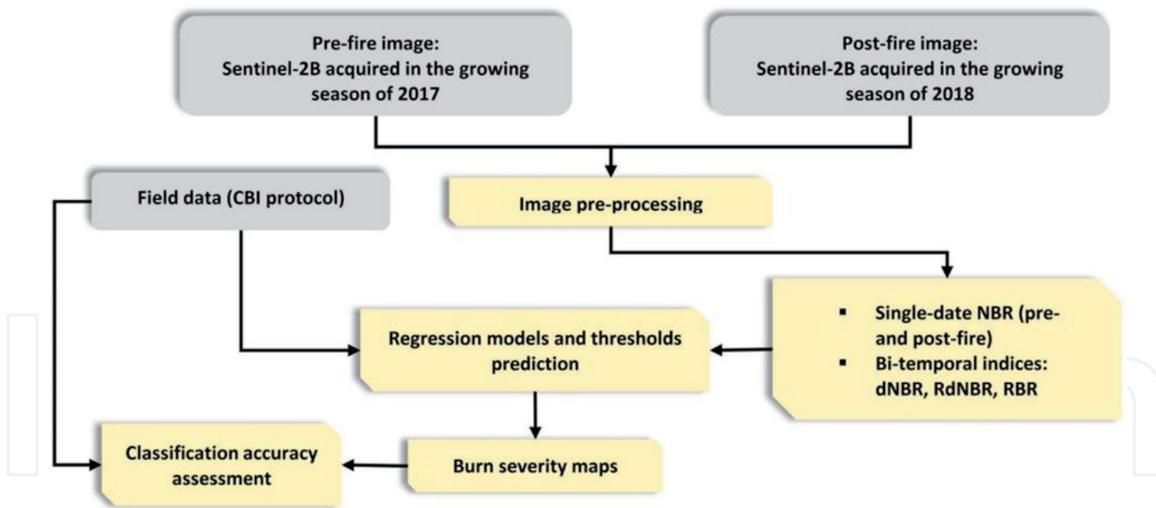
**Figure 5.** Developed workflow to retrieve burn severity maps from remote sensing data based on remote sensing indices (normalized burn ratio, NBR; differenced normalized burn ratio, dNBR; relative difference normalized burn ratio, RdNBR; relativized burn ratio, RBR) and field data (composite burn index, CBI).
