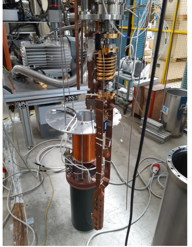
FIG. 1. View of the QUAX- a\gamma dilution refrigerator insert, instrumented with the resonant cavity (at the bottom) and amplification chain. In the background, the 8.1 T magnet with its countercoil is visible.
