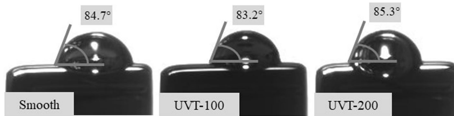
Fig. 5. Water droplets on the surfaces of the Ti6Al4V machined samples
