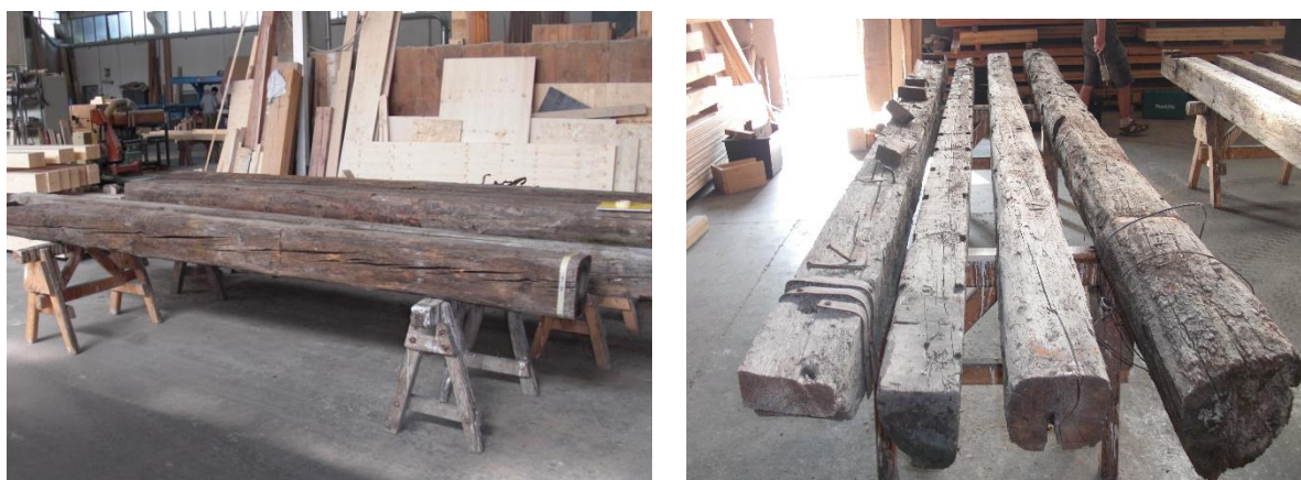
Figure 1: Timber beams ready to be tested at Bozza Legnami premises
