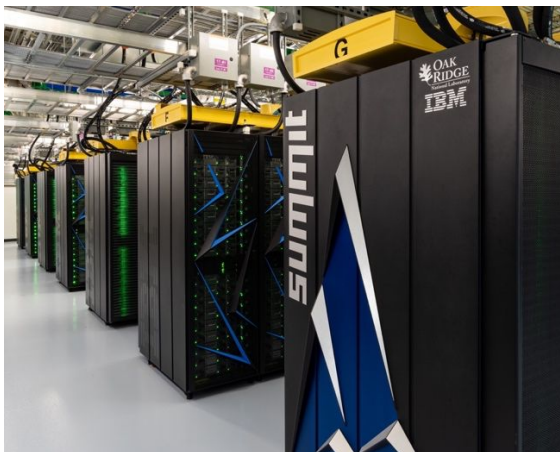
Fig. 14 – The Summit supercomputer, in operation at the Oak Ridge NL, US, was the fastest supercomputer in the world as of November 2018. (Carlos Jones/ORNL at Wikimedia Commons) With a measured power efficiency of 14.668 GFlops/watt it was also the 3rd most energy efficient in the world. Since 2020 it has been surpassed by Japanese Fujitsu Fugaku, capable of 415,5 PLFOPS.
