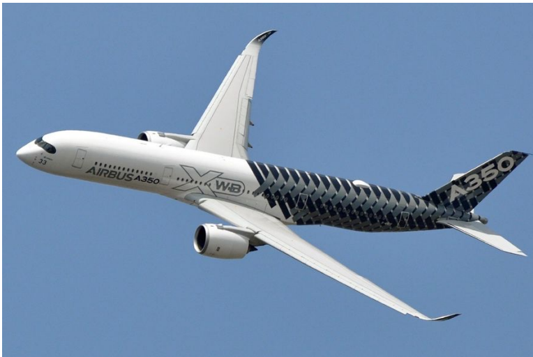
Fig. 10 – The Airbus A350, released in 2013, makes large use of composite materials in its structure and fuselage (Eric Salard in Wikimedia Commons)
