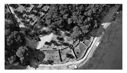
Figure 13: The Dražica sheepfold with nine enclosures. In the upper left corner of the photo, the dry stone wall terracing is visible – stones from the terraces became part of the single walls of the new sheepfold. The long dry stone wall on the left served as a tres – a wall along which the sheep were driven to the sheepfold. The parking lot probably served as a pregrajčić. The przgar is located in the middle (the round enclosure with vegetation) (2020).
