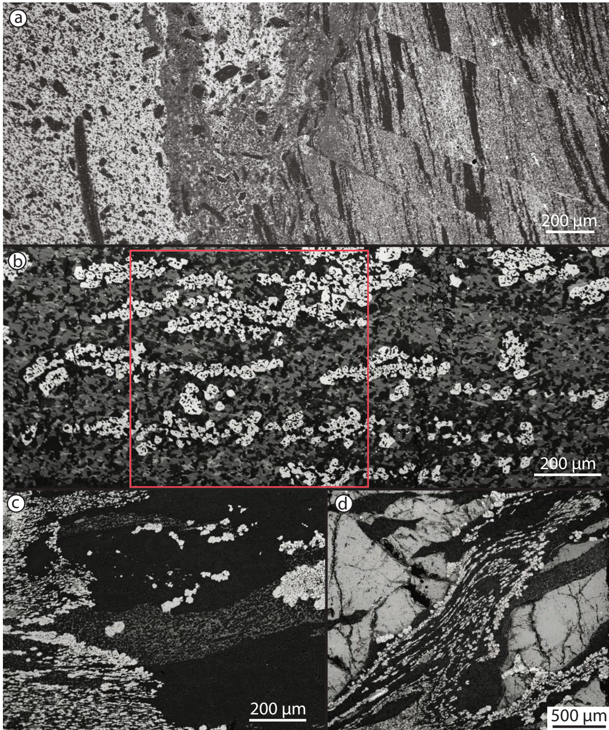
Figure 5. Backscattered electron images of pseudotachylyte: (a) late-stage pseudotachylyte with angular clasts in mylonitic host rock with abundant fractures (26.3550 S, 131.8432 E). (b) Dynamically recrystallized pseudotachylyte in sample F68. Minerals in greyscale from dark to bright are Qz, Pl, Kfs, Ky, Bt, and Grt. The red box indicates the mapped area for Fig. 7. (c) Un-sheared pseudotachylyte in a vein cutting through a plagioclase grain of the granulitic host rock showing dendritic overgrowth of garnet. In the left part of the image, the pseudotachylyte is finely grained and foliated (sample S5). (d) Injection vein preserves original flow banding, visible through the selective overgrowth of garnet (sample S5).
