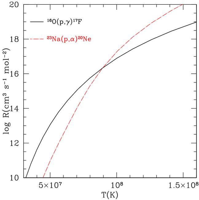
**Figure 1.** The rates of the  $^{16}\text{O}(p, \gamma)^{17}\text{F}$  and  $^{23}\text{Na}(p, \alpha)^{20}\text{Ne}$  reactions as a function of temperature, showing that for  $T \lesssim 10^8$  K oxygen is destroyed faster than sodium, whereas sodium is destroyed faster above this temperature.
