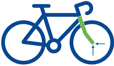
Fig. 3. Schematic of a bicycle and forces applied on the forks.
