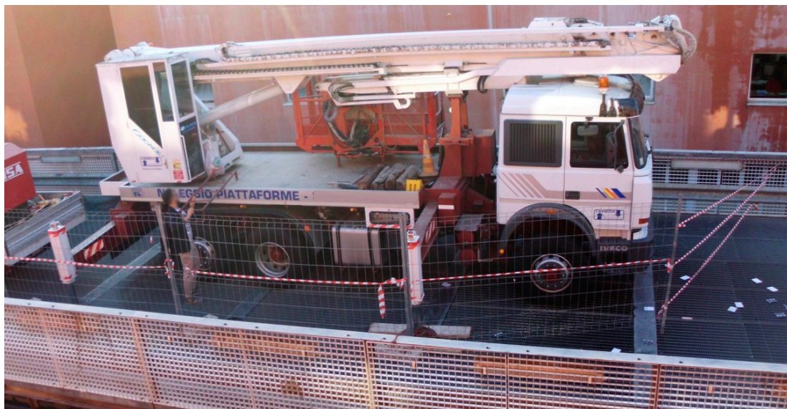
Figure 8. The truck elevator on the upper deck of the bridge.
