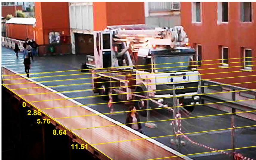
Figure 9. A frame of the camcorder video with the truck leaving the bridge. The transverse beams on the deck are used to obtain the position in the direction parallel to the longitudinal axis of the bridge.
