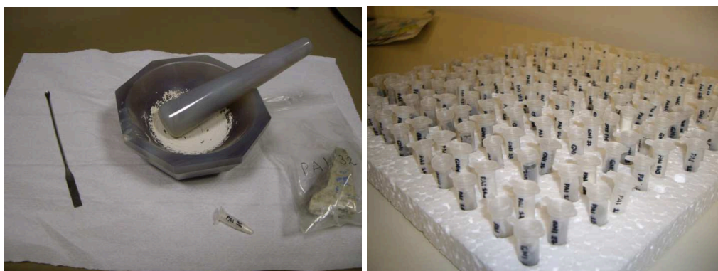
Figure 4.4: on the left: tools for the grinding of the samples: spatula, mortar with pestle, test tube, rock samples. on the right: the powdered samples.
