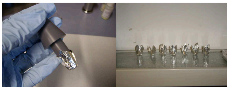
Figure 3.3 – on the left: plastic stencil for the creation of the vessels from the tin foil. On the right: capsules or vessels.
