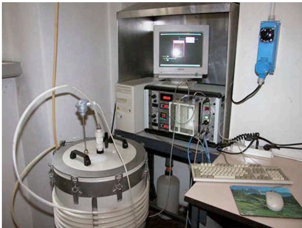
Figure 3.8 – the adiabatic fermenter used for composting test
