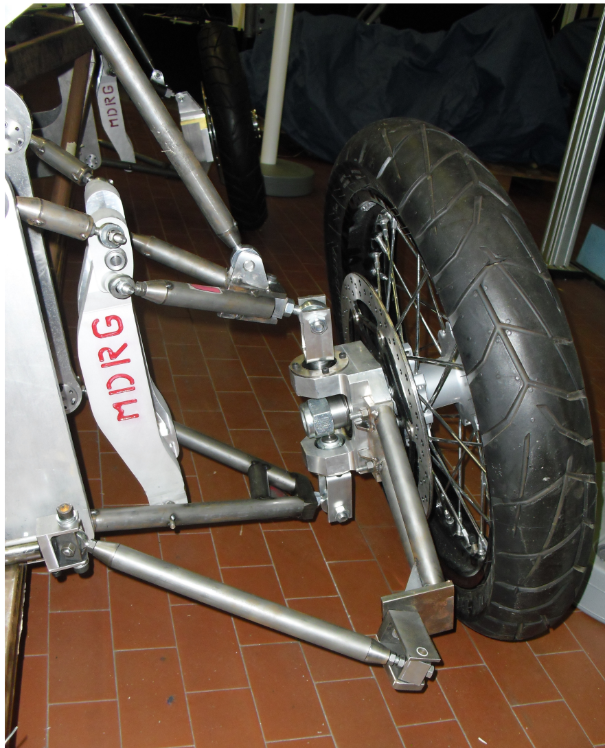
Figure 6.22: Suspension and track rod
