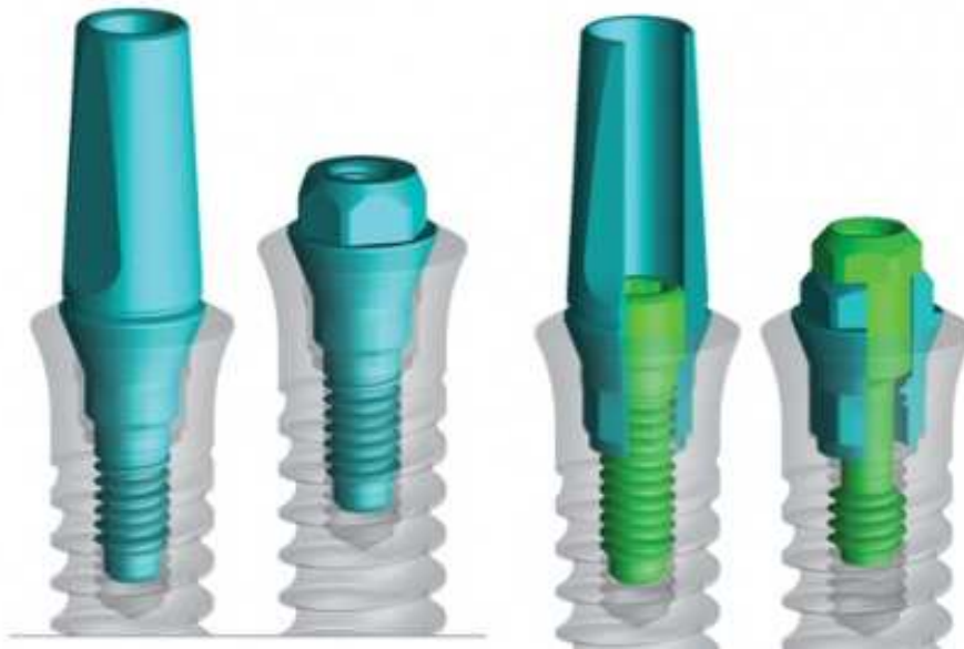
FIGURE 14 EXAMPLE OF CONNECTION BETWEEN FIXTURE AND CROWN ON PREMIUM KHONO TG: ABUTMENT FOR CEMENTED CROWN (ON THE LEFT) OR BALANCE BASE PILLAR FOR OVERDENTURES (ON THE RIGHT) AND HIS SCREWED RETENTION SYSTEM
