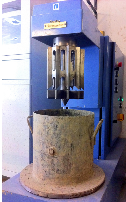
Figure 6-2. ConTec BML Viscometer 3.
