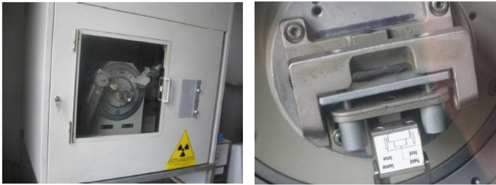
Figure 3-14. XRD – left: particular of the goniometer; right: sample holder.
