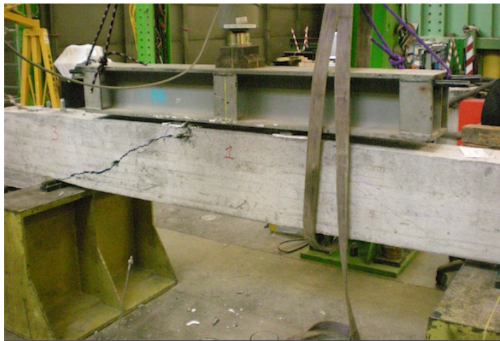
Figure 4-15. Shear failure - "B1" series.
