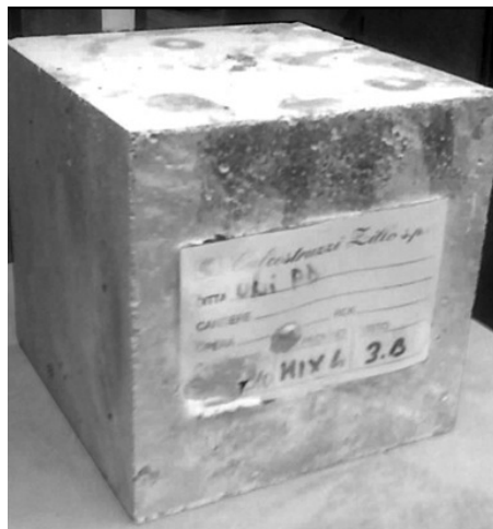
Figure 3-7. White powder outcrops on specimens after accelerated ageing treatment.
