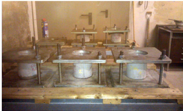
Figure 8-17. Water depth penetration test.
