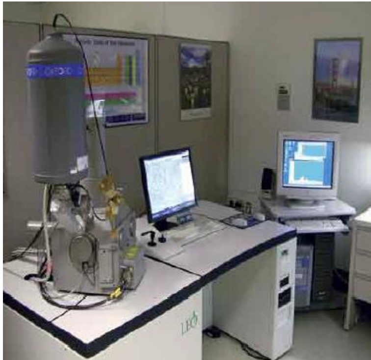
Figure 3-13. SEM – Scanning Electron Microscope, equipped with EDX.
