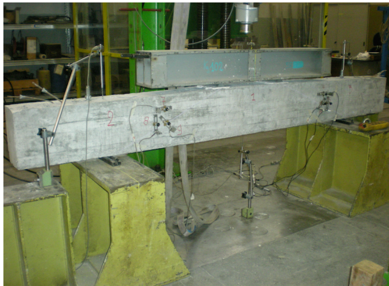
Figure 4-28. Instrumentation disposition - shear failure.
