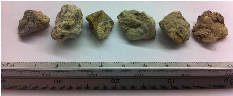
Figure 6-8. RA with high attached mortar content.
