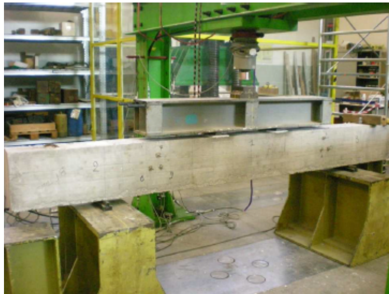
Figure 4-26. Four-point bending test.
