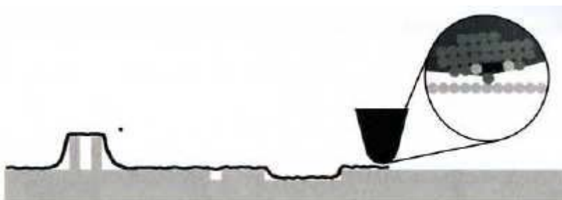
Figure 2-3 Resolution limits in a conventional STM instrument. Images of step walls and holes are distorted when their size is comparable to that of the tip apex
