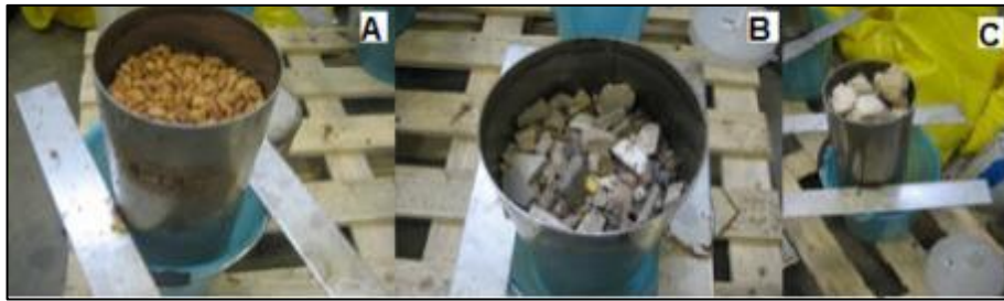
Figure 2.2 Three of the four materials used for the RD percolation test: brick 8-12mm (A), tiles 8-80 mm (B) porous refractory 8-100 mm (C).
