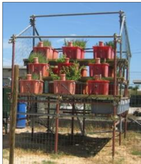
Figure 4.12 The phytodepuration system (CCW) experimented in 2012.
