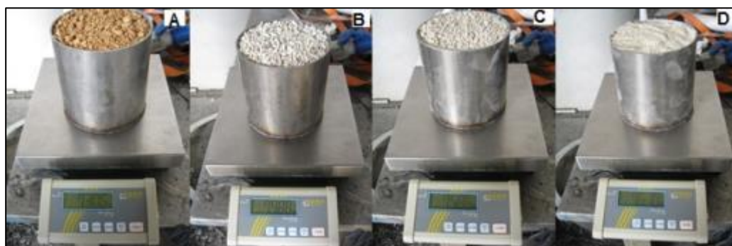
Figure 2.1 Four of the five materials used for the first percolation tests: brick 6-12mm (A), porous refractory 3-12mm (B), porous refractory 0-6 mm (C), porous refractory 0-3 mm (D)
