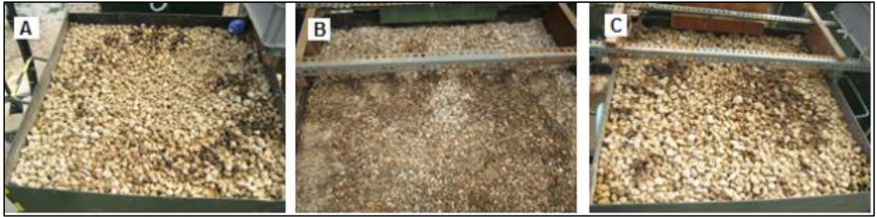
Figure 4.21 View of the top of some filters: A- filter with pumice and gravel; B- filter with gravel; C- filter with pumice.
