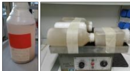
Figure 4.25 Pumice samples before and during stirring for the ammonium desorption test.
