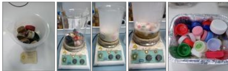
Figure 4.24 Removal of organic matter from the tops. The photos show the several phases from before (left) to after (right) the treatment.
