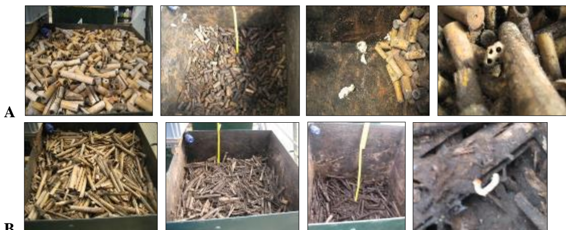
Figure 4.80 State of the bamboo (A) and giant reed (B) filters observed during the final surveys (2014).
