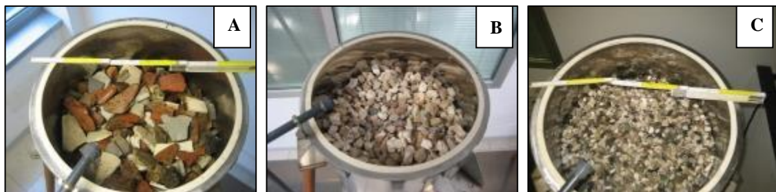
Figure 2.10 Filtering substrates: brick substrate used in F1(A); porous refractory substrate used in F2 and F3 (B); gravel used in F4 (C).
