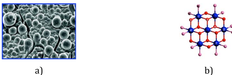
Fig. 1.9: a) Scanning electron microscopy (SEM) image of a cobalt phosphate (Co-Pi) film for electrocatalytic water oxidation; (72) b) edge-sharing molecular cobaltate cluster as the proposed model for the surface catalyst (73)
