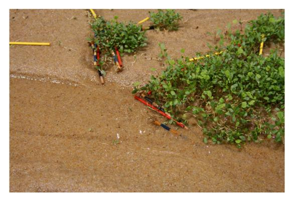
Figure 32: Example of interaction between LW and vegetation during a flood simulation.
