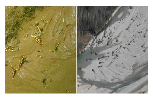
**Figure 74:** *Pieces of large wood stranded on a bar next to a big island in the flume (on the left) and on the Tagliamento River, in Italy (on the right).*
