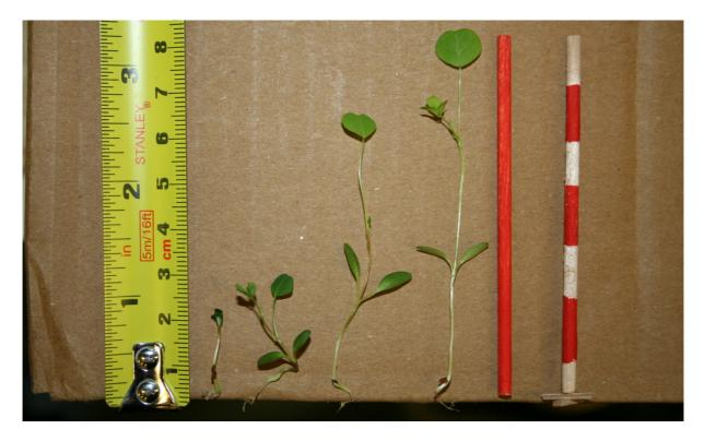
**Figure 31:** *Example of Alfalfa seeded and the dowels (with and without rootwad) used in the flume.*
