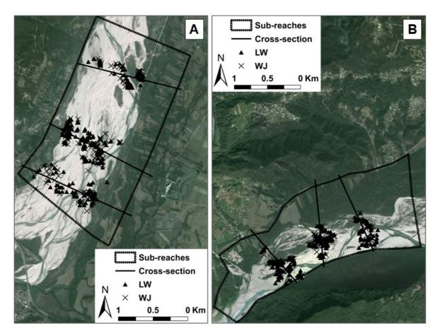
**Figure 14:** Localization of large wood (LW) and wood jams (WJ) in (A) Cornino and (B) *Flagogna sub-reaches in Tagliamento River.*
