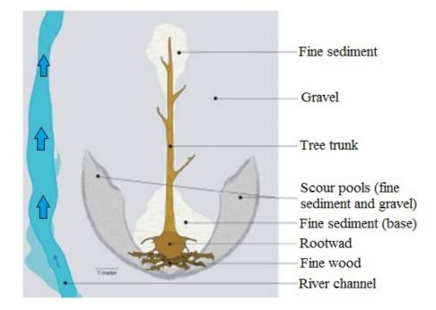
Figure 5: Typical spatial patterning of a deposited tree (after Francis et al., 2008).
