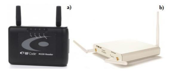
Figure 26: Mobile reader (a) and fixed reader (b) of the company RFCode Inc.
