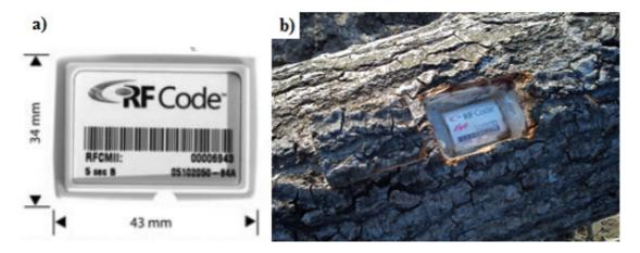
**Figure 27:** *Example of active RFID tag are those of the company RFCode Inc in which each tag is enclosed in shock resistant and splash resistant case that is 47-34-12 mm in size (a). Example of tag installation (b).*
