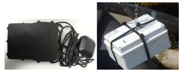
**Figure 29:** *Example of a LandAirSea's 3100-EXT passive GPS tracker (on the left) and its installation (on the right).*
