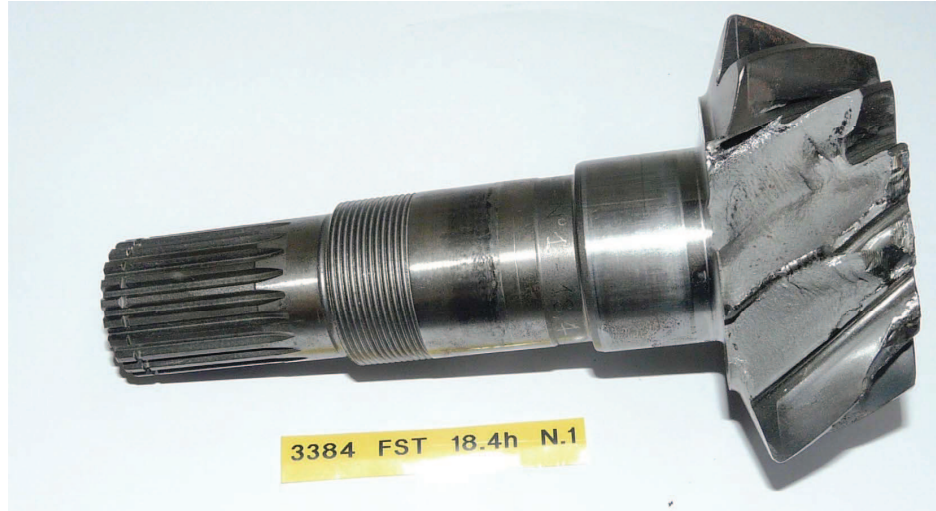
Figure 2.5: Failure of teeth of a bevel pinion (CT 3884).
