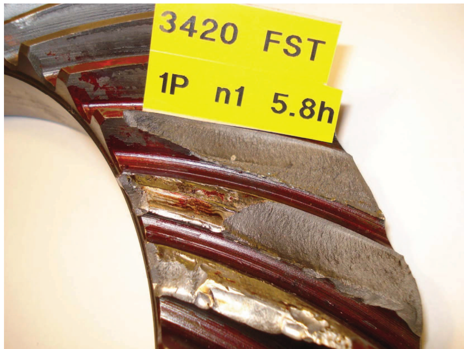
Figure 2.6: Failure of teeth of a bevel gear (CT 3884).
