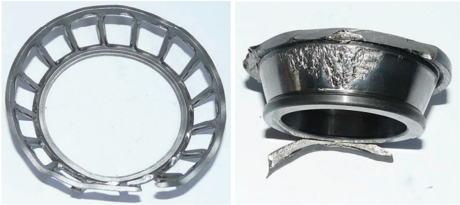
Figure 2.7: Failure of tapered roller bearing of bevel pinion (CT 3884).
