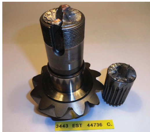
Figure 2.13: Failure of bevel pinion shaft on key slot (EST 3443).
