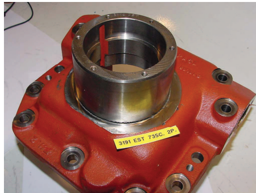
Figure 2.12: Failure of differential housing on fillet (EST 3191).
