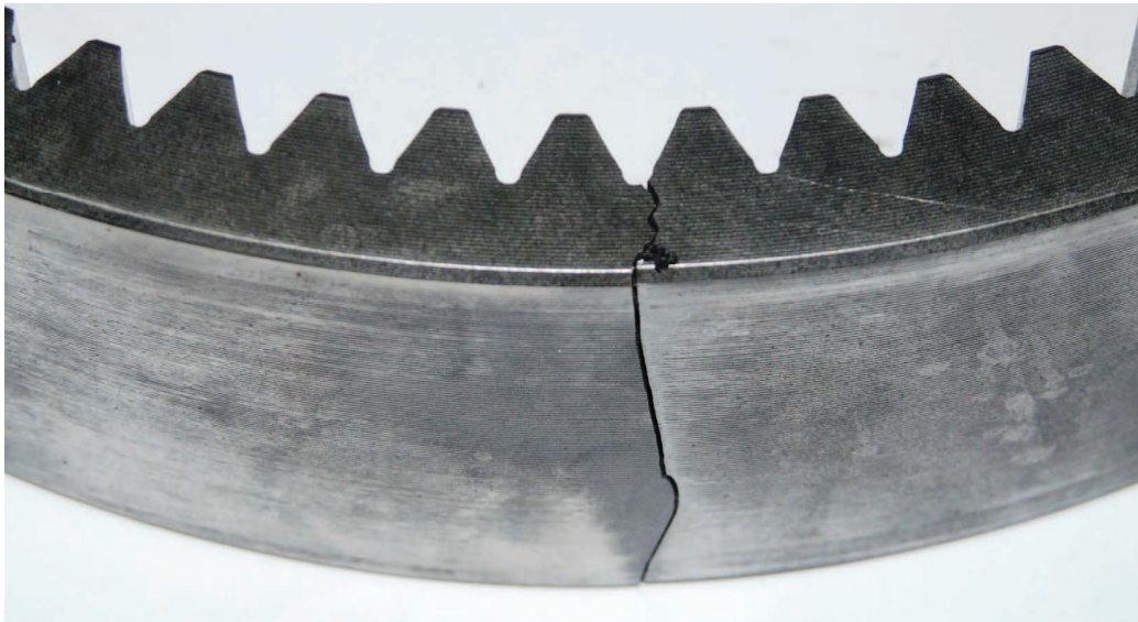
Figure 2.8: Failure by bending tooth root fatigue of the ring of a wheel hub drive (CT 3884).
