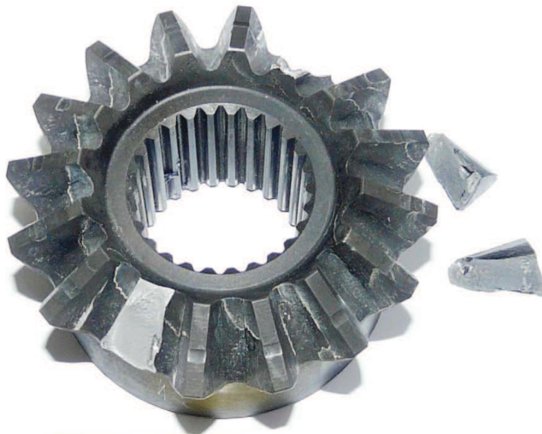
Figure 2.11: Failure of spider gear of differential (EST 3396).
