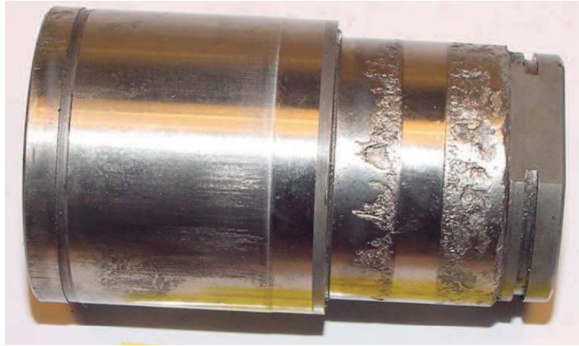
Figure 2.4: Pitting on planet pins (FST 3353).
