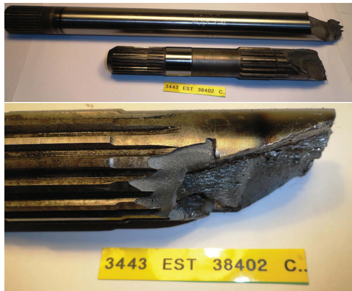
Figure 2.9: Failure of the axle shaft on spline (EST 3443).
