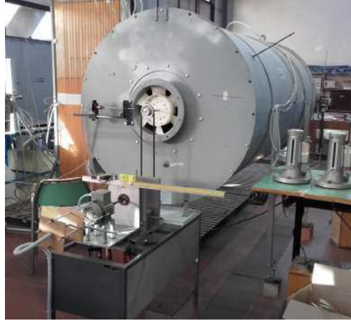
Figure 20: The torque crane used to measure the shaft torque T_a , installed on the medium-size rig.
