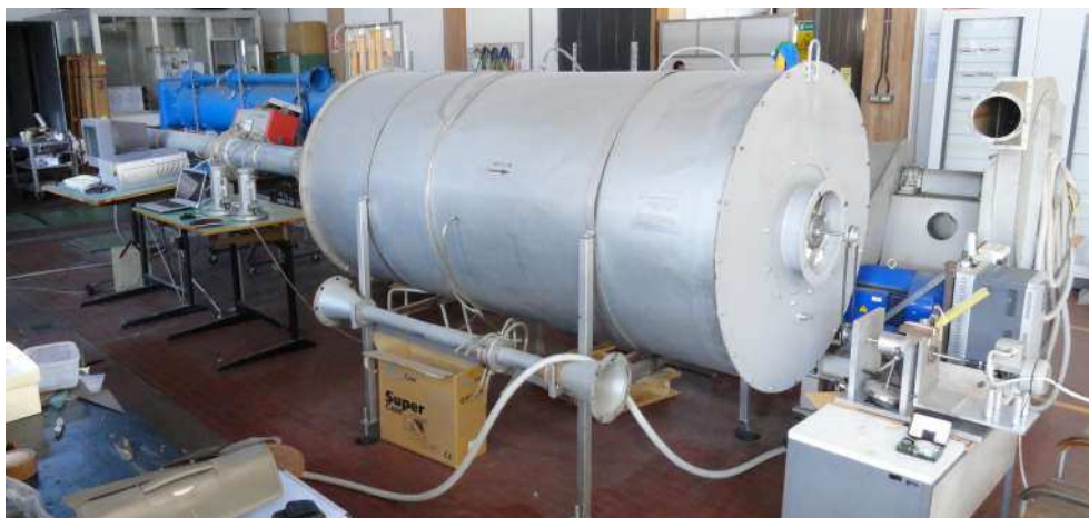
Figure 8: The medium-size inlet-chamber fan testing rig installed at the Laboratorio di Macchine Aerauliche e Termiche in Padova, Italy. The fan under test is positioned at the chamber exit (right side of the picture).
