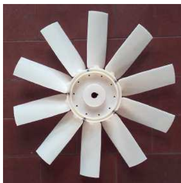
Figure 21: A 315 mm arbitrary-vortex 3D printed rotor with \nu = 0.32 .
