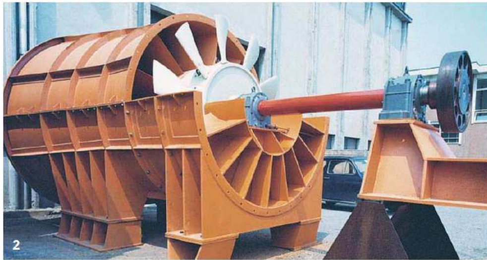
Figure 7: A PRS fan installed in a steel production plant in Italy, for conglomerate cooling purpose before entering the furnace (reproduced by courtesy of Boldrocchi Spa).
