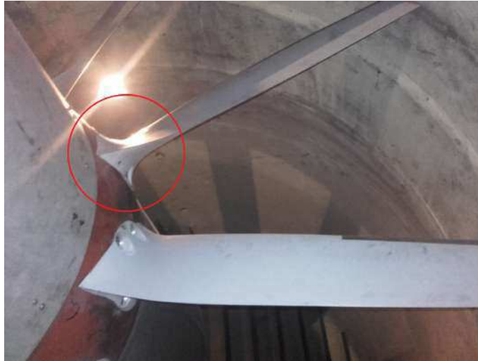
Figure 46: Particular of the blade attachment system of the 4.2 m Von Karman Institute wind tunnel CR fan.
