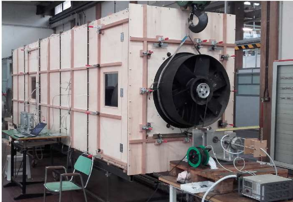
Figure 19: The large test rig (end-wall chamber side) and related scheme (adapted from [9]). The picture shows a 800 mm PR fan under test.
