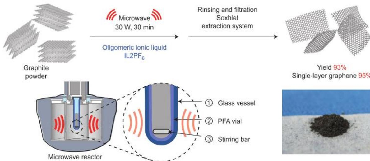
Figure 1.6 Microwave-assisted liquid-phase exfoliation of graphite in ionic liquids. (ref. 20c)
