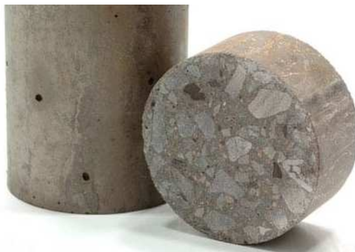
Fig. 2.6 Concrete sample at the mesoscale level.
