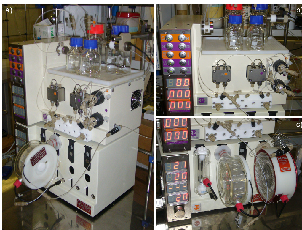
Figure 3.1: a) fully assembled Vapourtec R4 continuous flow platform and particulars of b) pumping module and c) heating module bearing various reactor modules.
