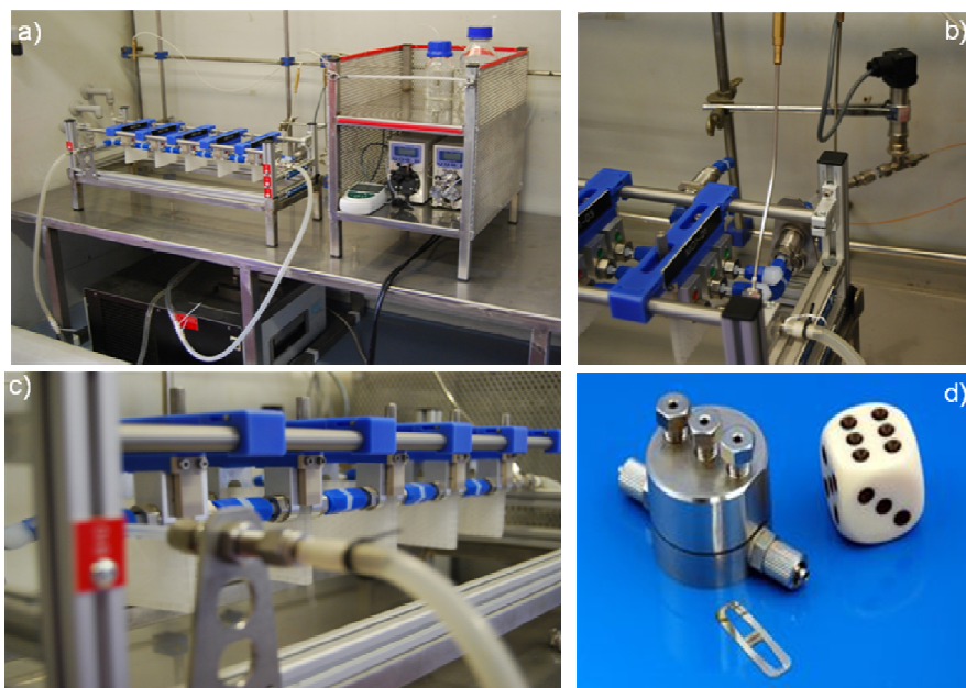
Figure 3.6: examples of continuous set-ups and support apparatus: a) a Low Flow complete reactor assembly involving also pumping, heating and controlling units. b) on-line probes for temperature and pressure monitoring. c) fluidic modules interconnected through Swagelok fittings and d) an IMM micromixing device. 9
