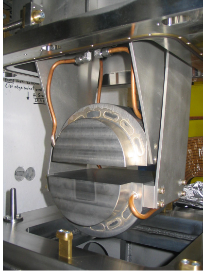
Figure 3.9: Thick copper slits placed along FRS beam line.
