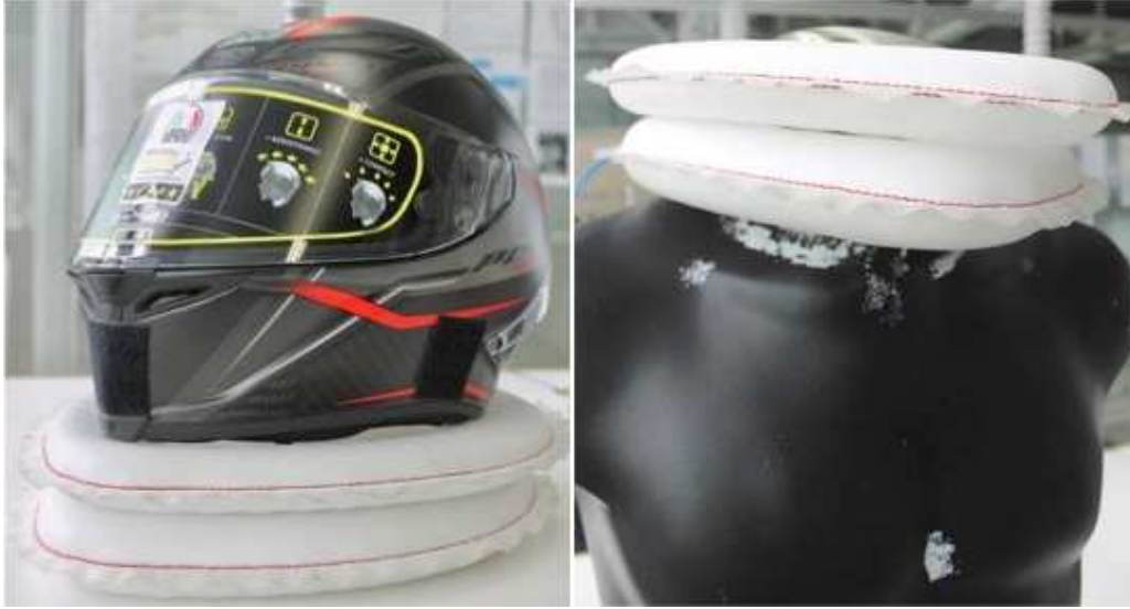
Figure 8.22 The contact between the helmet and airbag system as neck protector (left) and the position of the airbag layers around neck while inflated (right)
