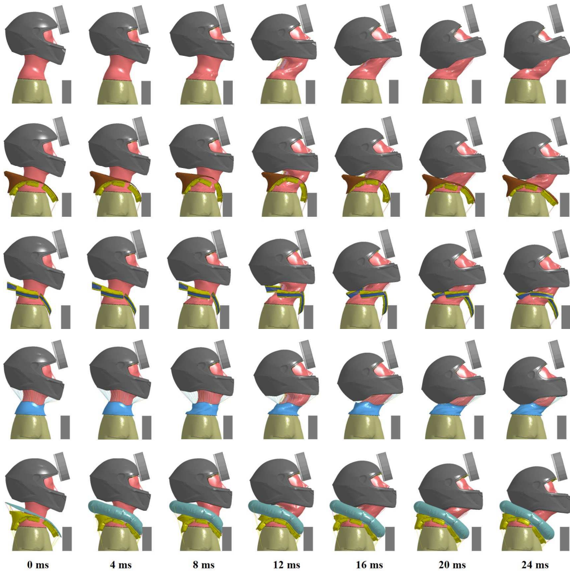
Figure 9.8 Time-lapse of the response of the ATD model with different neck protective systems for case 1
