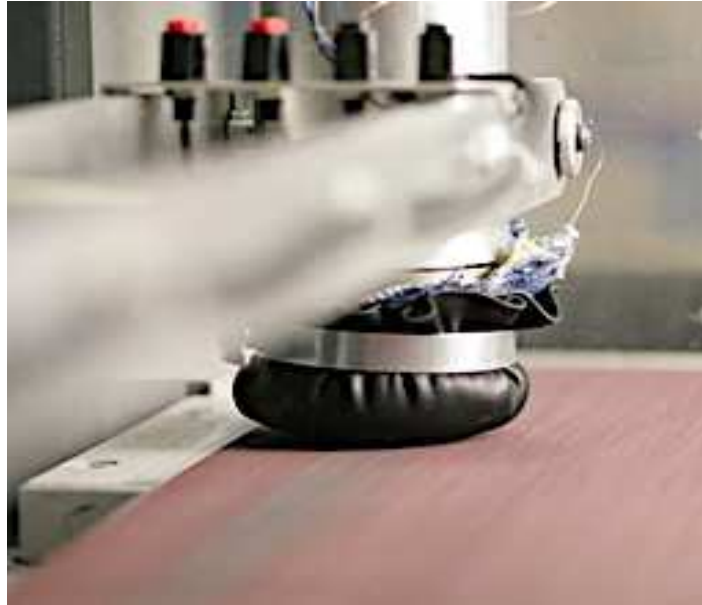
Figure 6.7 The test specimen of the leather garment mounted on the hinged arm of the Cambridge machine for the impact abrasion test
