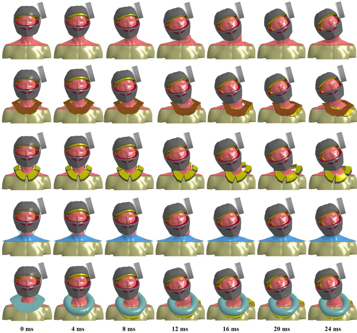
Figure 9.12 Time-lapse of the response of the ATD model with different neck protective systems for case 3
