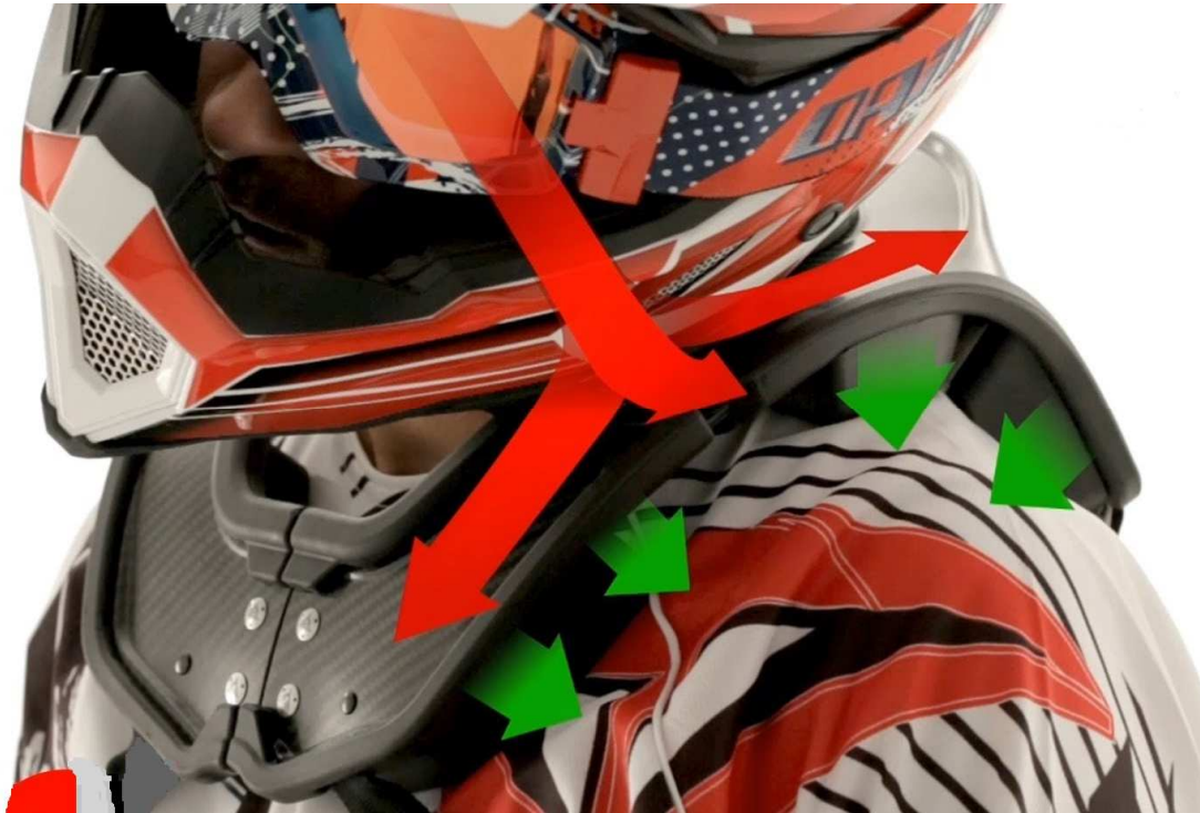
Figure 3.8 The principle of Hybrid Neck Brace [ www.dainese.com ].
