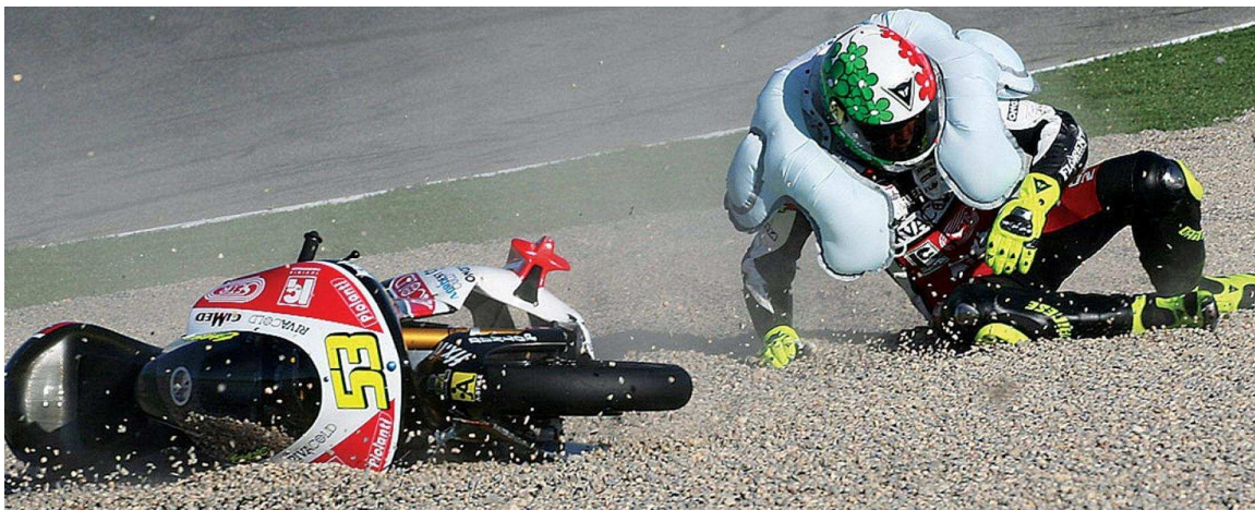
Figure 3.9 Mechanically triggered airbag system with physical connection to the motorcycle [www.dainese.com]
