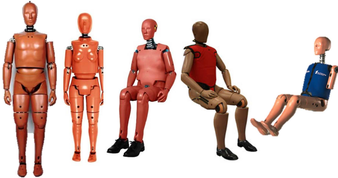
Figure 5.1 Different types of crash dummies: (from left to right) Hybrid III 50 th Male Pedestrian, Hybrid III 5 th Female Pedestrian, BioRID II 50 th Male Rear Impact, THOR 50 th Male Frontal Impact, SID IIs 5 th Female Side Impact (adapted from www.humanetics.com )
