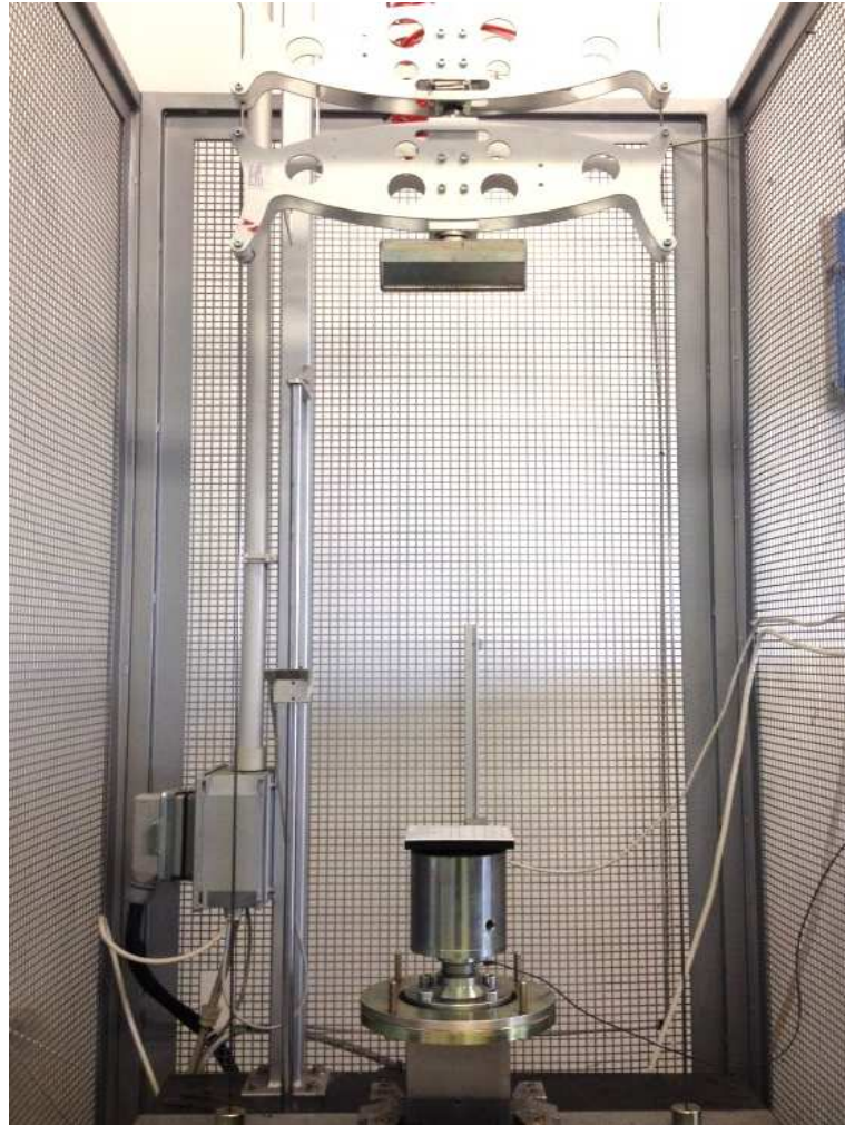
Figure 6.3 The experimental set-up of a drop weight impact tester for the impact test
