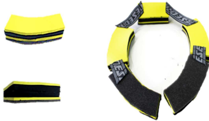
Figure 8.10 The complete structure of the soft brace (right), which has been designed as layers of different types of foams: two layers of Poron XRD foam, one layer of polyurethane comfort foam and one layer of nitrile butadiene rubber (NBR) placed in between the two Poron layers (left).
