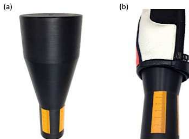
Figure 6.11 (a) A rigid test cone for the restraint test and (b) the performance of the restraint test using the test cone
