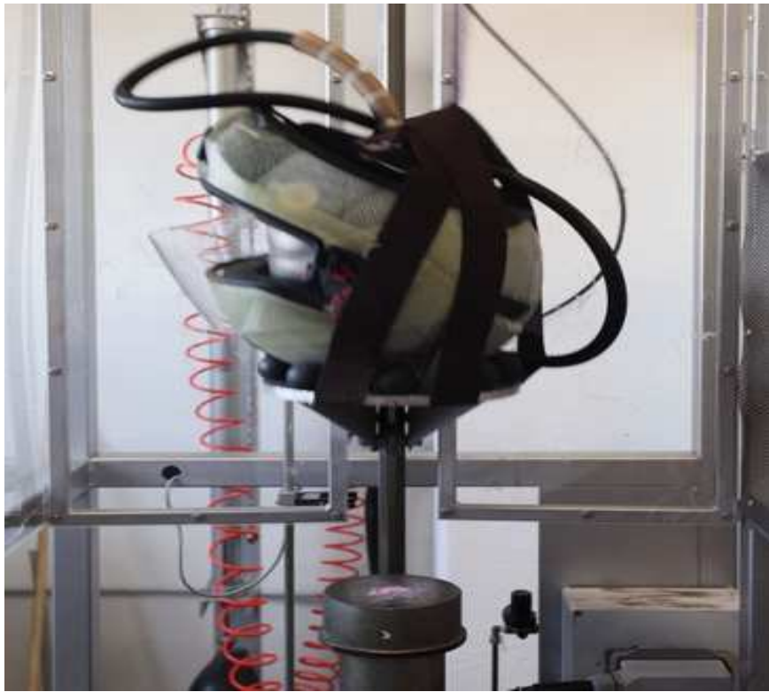
Figure 6.4 The experimental set-up of headform drop assembly [Reproduced from www.mavet.it ]
