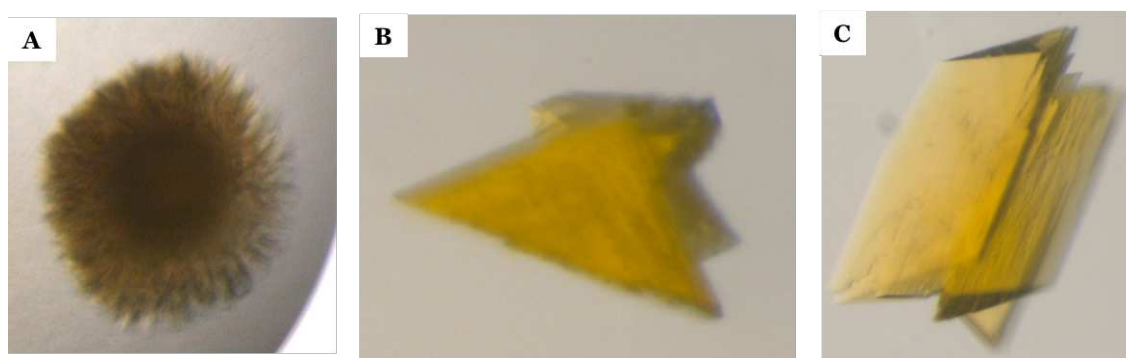
Figure 80. CtOYE crystals optimization: (A) first crystal hits obtained with N-tagged CtOYE; (B) and (C) crystals obtained after His-tag removal using micro-seeding and Fos-choline as additive.
